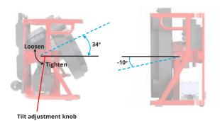
For confined space rescue operations, you can place the ventilator directly on top of a manhole. Tilt range from -90 to +90 degrees. Note that those positions can direct airflow downward or upward
