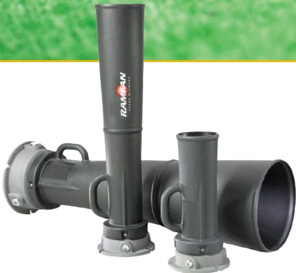
Safe for use in explosive atmospheres. Venturis are powered by compressed air or saturated steam. They operate on the Venturi principle of using small volumes of high velocity air (from a compressed source) pushing the air through the cone body creating entrained air (pulling action), which induces large volumes of low velocity air through the cone and out the air diffuser.
