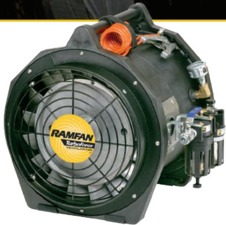
Pneumatic, explosion-proof blowers for use in hazardous locations. High strength anti-static housing with integrated duct adapters. Compressed air does not enter the airstream. Complete with filter, motor lubrication, exhaust muffler, air control valve and static grounding cord.
