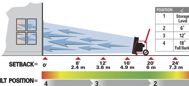
Note: Output changes as setback from the opening changes. Single door airflow is per AMCA 240-6 testing. This data derives from 0° static pressure. Test results from fan set back 5.5m at 12° tilt and 3,684 rpm. Real world results will be substantially reduced by structure back-pressure.
