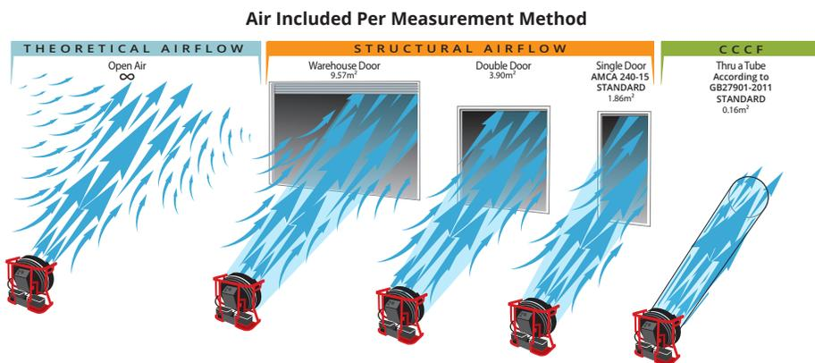
During the ventilation process, airflow from the fan will create large amounts of entrained air. Entrained air is the natural effect from the high velocity airflow creating friction with the air next to it, thereby pulling the air into the flow path. While measuring airflow, entrained air that goes through the opening must be included in the airflow calculation to reflect realistic ventilation obtained by the fan.
