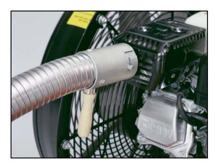
A new and improved exhaust diverter for the RAMFAN PPV Turbo Blowers is now available. The newly redesigned exhaust diverter has been improved for rerouting unwanted carbon monoxide away from the work area. The new diverter hose has increased in diameter and length to 2" x 12' for improved performance and can quickly couple to additional hoses in increments of 12' to divert CO fumes even further away. Call now to place your order.
