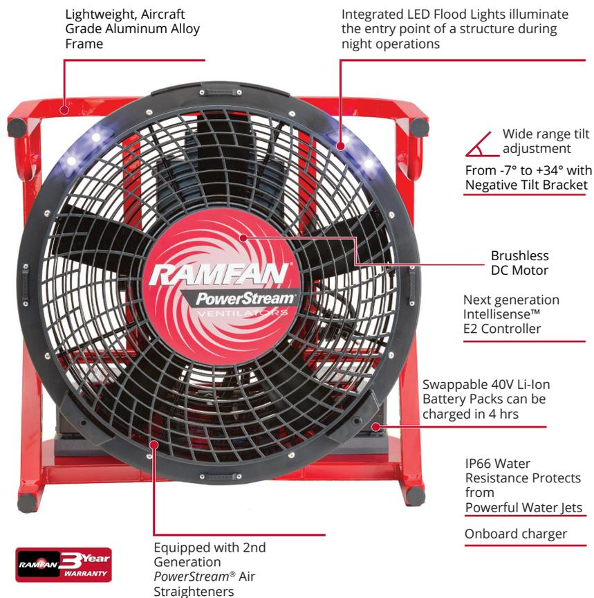
*Note: Output changes as setback from the opening changes. Single door airflow is per AMCA 240-15 testing. This data derives from 0" static pressure. Real world results will be substantially reduced by structure backpressure. EX50Li is tested at 13.5 ft (4.1 m) setback at 12.7° tilt and 2924 rpm on AC Power Supply and tested at 14 ft (4.3 m) setback at 9° tilt and 3045 rpm on DC Power Supply.*
