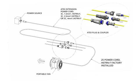
The Power Extension Cables described here are intended for use in Explosive Atmospheres in accordance within the limitation of the ratings. It is the user's responsibility to determine the suitability of the equipment for the intended purpose.
